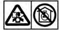
The exhaust gases are dangerous Do not use in a poorly-ventilated area
